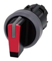
Selector switch, illuminable, 22 mm, round, plastic with metal front ring, red, selector switch, short, 3 switch positions I-O<II, left latching, right momentary contact type, actuating angle 2x45°, 10:30h/12h/13:30h, with laser labeling, upper case and lower case, always upper case at the beginning of the word
