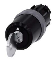
key-operated switch Siemens, 22 mm, round, plastic with metal front ring, lock number SSG10, with 2 keys, 3 switch positions I-O-II, latching, actuating angle 2x45°, 10:30h/12h/13:30h, key removal O+I, with laser labeling, upper case and lower case, always upper case at beginning of line
