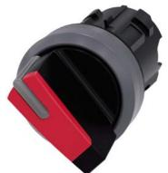
Selector switch, illuminable, 22 mm, round, plastic with metal front ring, red, selector switch, short, 2 switch positions O-I, latching, actuating angle 90°, 10:30h/13:30h, with laser labeling, inscription or symbol Customer-specific selection with SIRIUS ACT configurator (CIN)
