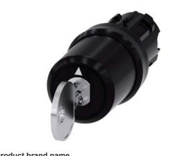
key-operated switch Siemens, 22 mm, round, plastic, lock number SSG10, with 2 keys, 3 switch positions I>O<II, momentary contact on the left, latching on the right, actuating angle 2x45°, 10:30h/12h/13:30h, key removal O+II Z=50-unit packaging
