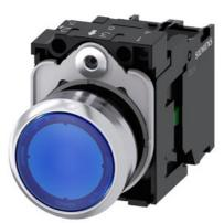
Illuminated pushbutton, 22 mm, round, metal, shiny, blue, pushbutton, flat, momentary contact type, with holder, 1NO, LED module with integrated LED 230 V AC, screw terminal, Z=20-unit packaging
