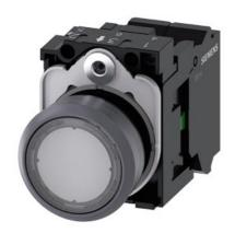
Illuminated pushbutton, 22 mm, round, plastic with metal front ring, clear, pushbutton, flat, momentary contact type, with holder, 1NO, LED module with integrated LED 24 V AC/DC, spring-type terminal, with laser labeling, inscription or symbol Customer-specific selection with SIRIUS ACT configurator (CIN)
