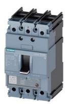
circuit breaker 3VA5 UL frame 125 breaking capacity class M 35kA @ 480 V 3-pole, line protection TM230, FTAM, In=40A overload protection Ir=40A fixed short-circuit protection Ii=5...10 x In UL489 SB (naval), 50 deg. cel. cable connection on both sides
