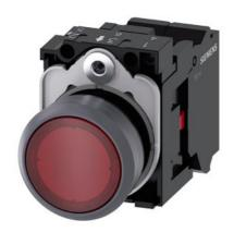
Illuminated pushbutton, 22 mm, round, plastic with metal front ring, red, pushbutton, flat, momentary contact type, with holder, 1NC, LED module with integrated LED 24 V AC/DC, spring-type terminal, with laser labeling, lower case
