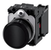
Pushbutton, 22 mm, round, plastic, black, pushbutton, flat, momentary contact type, with holder 1 NC, screw terminal, with laser labeling, inscription or symbol Customer-specific selection with SIRIUS ACT configurator (CIN)
