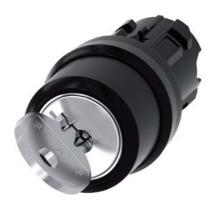
RONIS key-operated switch, 22 mm, round, plastic, lock number SB30, with 2 keys, 2 switch positions O-I, latching, actuating angle  $90^\circ, 10:30h/13:30h,$  key removal O, possible special locks: SB31, 421, 455, with laser labeling, upper case and lower case, always upper case at the beginning of the word
