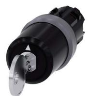
key-operated switch Siemens, 22 mm, round, plastic with metal front ring, lock number SSG10, with 2 keys, 3 switch positions I>O<II, momentary contact on the left, latching on the right, actuating angle 2x45°, 10:30h/12h/13:30h, key removal O+II, with laser labeling, upper case and lower case, always upper case at beginning of line
