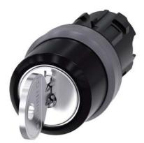
RONIS key-operated switch, 22 mm, round, plastic with metal front ring, lock number SB30, with 2 keys, 3 switch positions I-O<II, left latching, right momentary contact type, actuating angle 2x45°, 10:30h/12h/13:30h, key removal I, possible special locks: SB31, 421, 455, with laser labeling, upper case and lower case, always upper case at beginning of line
