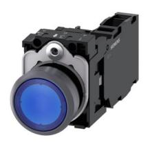
Illuminated pushbutton, 22 mm, round, plastic with metal front ring, blue, pushbutton, flat, momentary contact type, with holder, 1 NO+1 NC, LED module with integrated LED 230 V AC, screw terminal, with laser labeling, inscription or symbol Customer-specific selection with SIRIUS ACT configurator (CIN)
