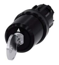
Key-operated switch BKS, 22 mm, round, plastic, special lock, with 2 keys, 3 switch positions I-O<II, latching on the left, momentary contact type on the right, actuating angle 2x45°, 10:30h/12h/13:30h, key removal I, Note: BKS locking systems E1 - E25 supplied without key
