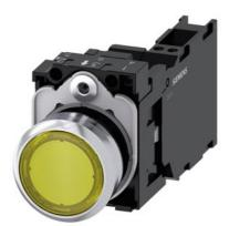
Illuminated pushbutton, 22 mm, round, metal, shiny, yellow, pushbutton, flat, momentary contact type, with holder, 1 NO+1 NC, LED module with integrated LED 24 V AC/DC, spring-type terminal, Z=20-unit packaging
