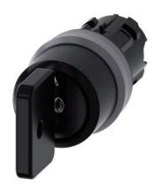
Key-operated switch O.M.R, 22 mm, round, plastic with metal front ring, lock number 73034, black, with 2 keys, 3 switch positions I-O-II, latching, actuating angle 2x45°, 10:30h/12h/13:30h, Key removal I+O+II, with laser labeling, upper case
