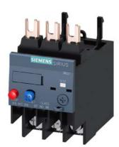
Overload relay 30...36 A Thermal For motor protection Size S0, Class 10 Contactor mounting Main circuit: Ring cable lug Auxiliary circuit: ring cable lug Manual-Automatic-Reset
