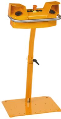
Preventa XY2, Two-hand control station with pedestal, orange, 2 push buttons 1 NO + 1 NC, 1 emergency stop push button 2 NC, pre-wired terminal block
