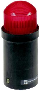
Harmony XVDLS, Monolithic tower light, plastic, red, Ø45, flashing, integral flash discharge tube 1 joule, 230 V AC
