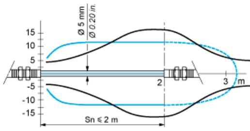
Excess Gain Curves (Ambient temperature:  $\pm 25\text{ }^{\circ}\text{C}$ )
