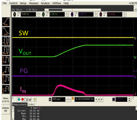
(5) Inrush Current Ta=25°C V_{IN}=6.0V , V_{SW}=V_{IN} \rightarrow 0V , V_{SHDN}=0V
