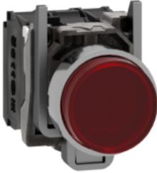
Illuminated push button, Harmony XB4, red flush, 22mm, spring return, plain lens, screw clamp terminals, 1NO + 1NC, 24V
