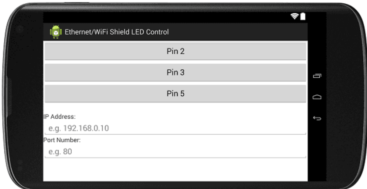
The Android app you can use to control the Arduino's pins through the WiFi or Ethernet Shield.
