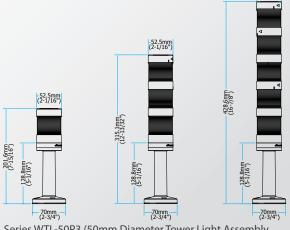
Series WTL-50P3 (50mm Diameter Tower Light Assembly with Direct Mount Base)
