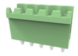
PCB connector Rated current: 8 A Rated voltage: 300 V Pitch: 3.81 mm Mounting: Wave soldering
