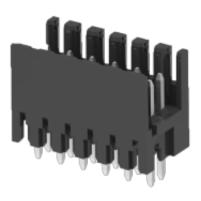
PCB connector Rated current: 7 A Rated voltage: 150 V Pitch: 3.5 mm Mounting: Reflow soldering
