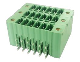
PCB connector Rated current: 8 A Rated voltage: 300 V Pitch: 3.5 mm Mounting: Wave soldering
