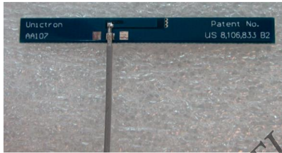
Figure 8-1. 2.4GHz PCB Antenna
