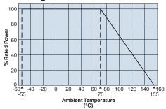
For resistors operated at an ambient temperature of 70°C or above, a power rating shall be derated in accordance with the above derating curve.
