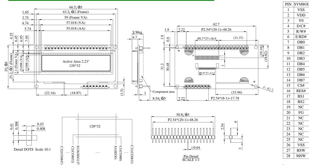
The non-specified tolerance of dimension is  $\frac{1}{2}$   $\hat{\mathbf{0}}$  3 mm.
