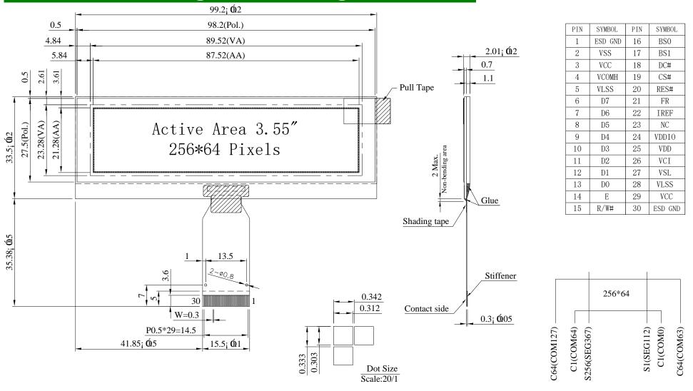
The non-specified tolerance of dimension is i **Q**3mm.
