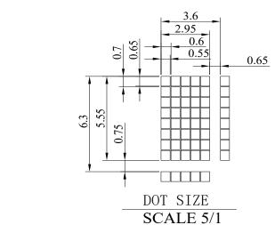
The non-specified tolerance of dimension is i 03 mm.
