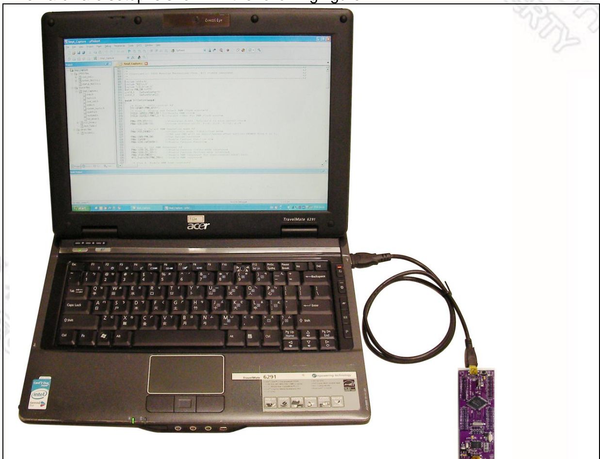
Figure 4-1 NuTiny- SDK-NUC220 Hardware Setup
