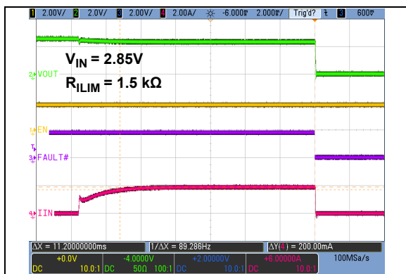
FIGURE 2-3: Overcurrent Fault Response Delay Time.
