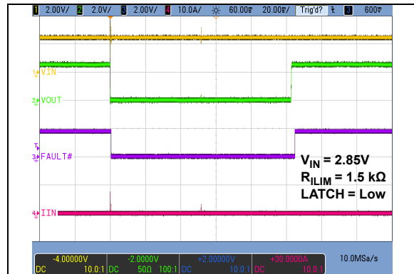
FIGURE 2-16: Output Recovery from Short Circuit.
