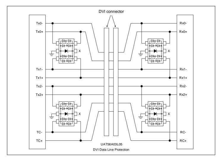
Electrostatic Discharge Protection Devices UAT56A03L05
