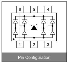
Electrostatic Discharge Protection Devices UAT56A03L05
