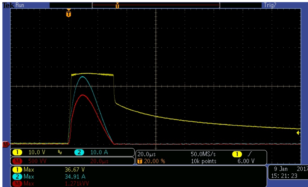
Figure 6. TVS3300YZF Surge Test Waveform
