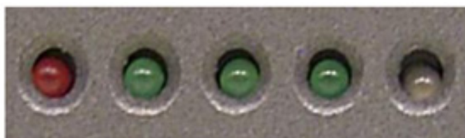
Red (Power) Green (Storage access) Green (RF data transfer) Green (RF link) Blue (GPS Operation)
