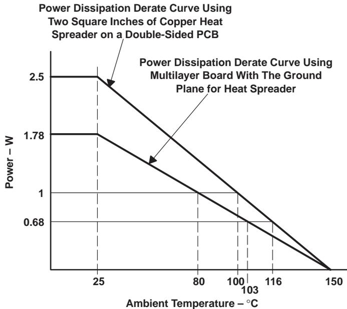
NOTE: These curves are to be used for guideline purposes only. For a particular application, a more specific thermal characterization is required.
