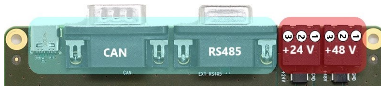
Figure 3: Power; Communication and USB-C connectors of TMCM-BB1
