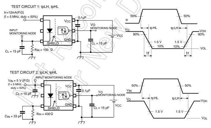
The PROBE and JIG capacitances are included in C<sub>L</sub>. (P.G): Pulse Generatior
