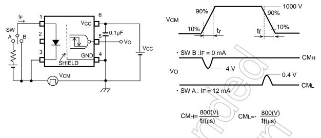
Note: CML (CMH) is the maximum rate of fall (rise) of the common mode voltage that can be sustained with the output voltage in the low (high) state.
