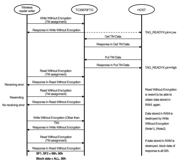
Figure 4-31 Sequence of resending Read Without Encryption
