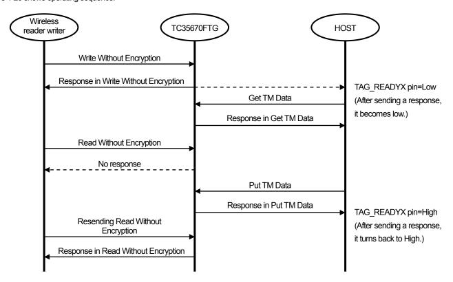
Figure 4-26 Operating sequence in Through mode
