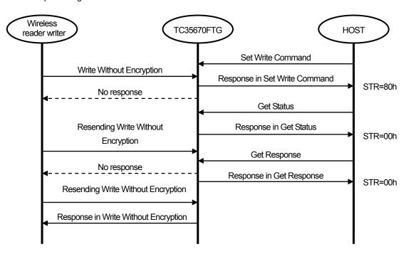
Figure 4-25 command processing sequence of wired interface
