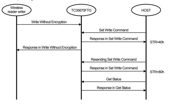
Figure 4-24 Command processing sequence of wireless interface
