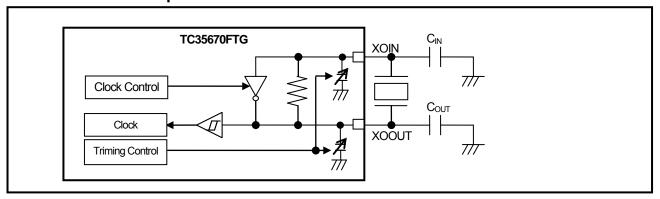
Figure 4-13 Crystal oscillator connection example
