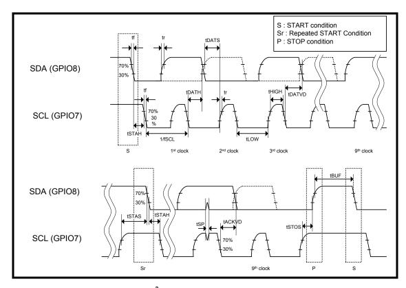
Figure 9-3 I<sup>2</sup>C Interface Fast mode Timing diagram
