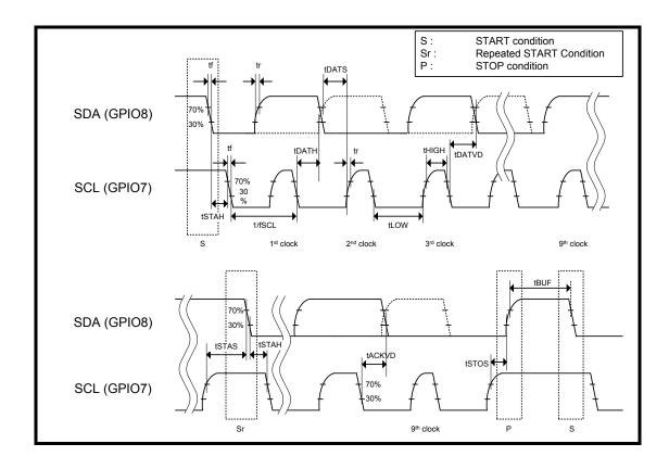
Figure 9-2 I<sup>2</sup>C Interface Normal mode Timing diagram
