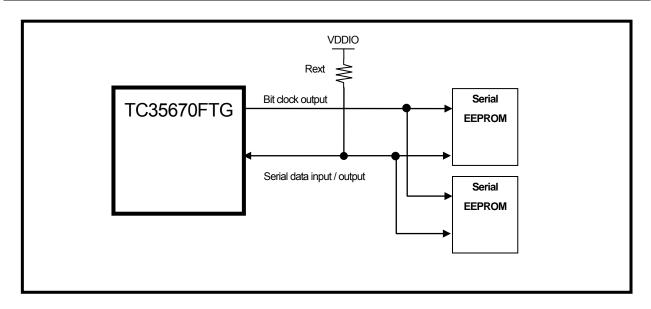
Figure 4-9 Connection example for serial EEPROM with I<sup>2</sup>C-bus interface (CMOS output)
