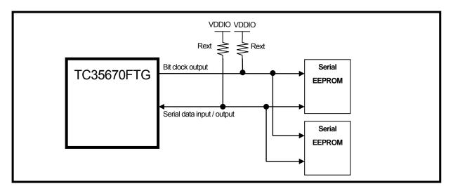
Figure 4-8 Connection example for serial EEPROM with I<sup>2</sup>C-bus interface (Open-drain output)
