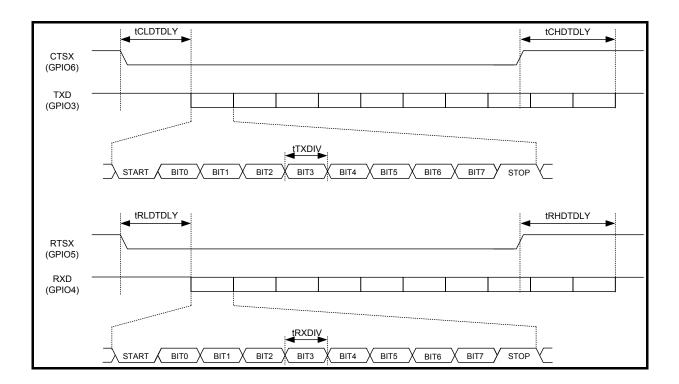
Figure 9-1 UART Interface Timing Diagram
