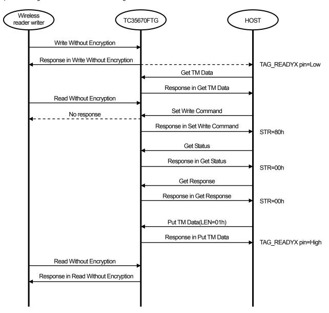
Figure 4-30 Sequence of usage of Set Write Command in Through mode
