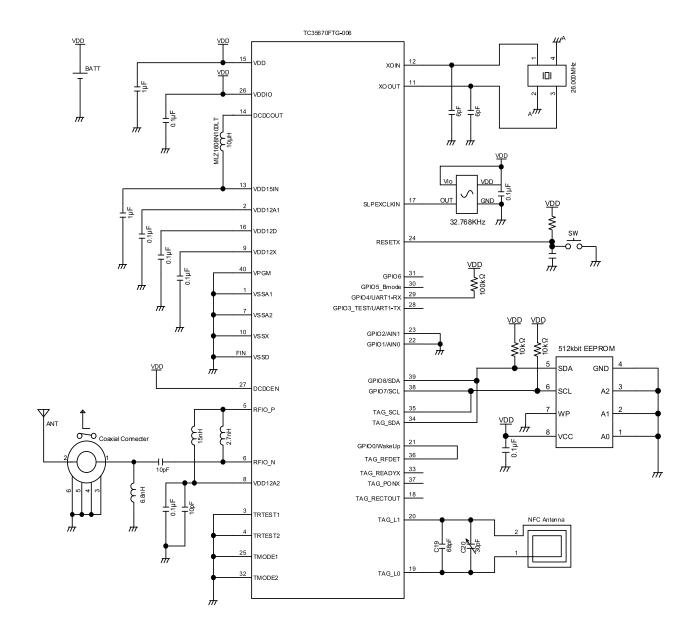
Figure 10-2 Example of TC35670FTG system configuration (Stand-alone)
