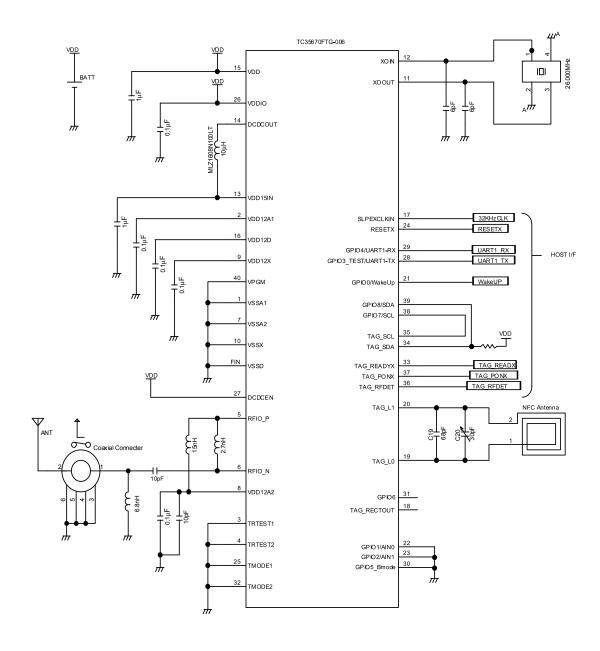
Figure 10-1 Example of TC35670FTG system configuration (HOST CPU connection)
