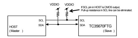
Figure 4-20 Connection example in usage of TAG-I<sup>2</sup>C mode
