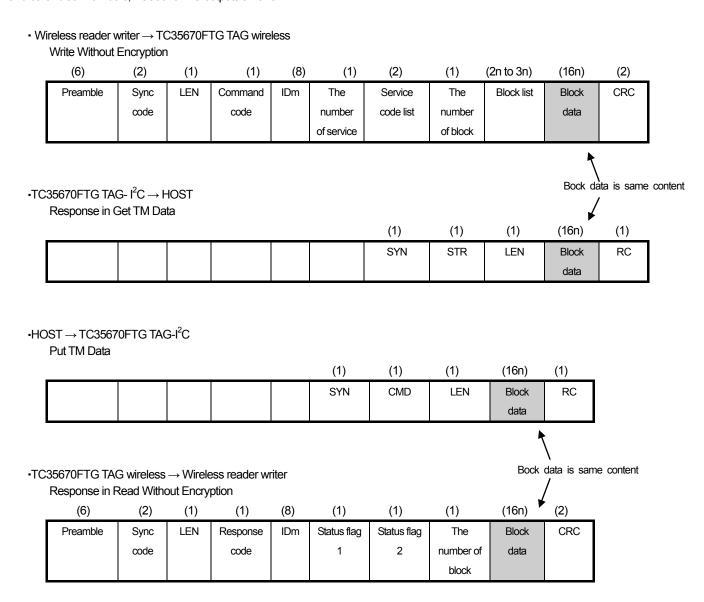
Figure 4-27 The explanation of packet in Through mode
