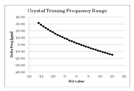
Figure 4-14 Trimming frequency range example
