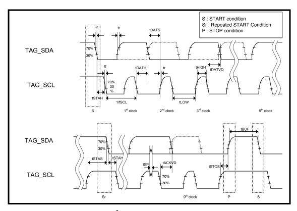
Figure 9-5 I<sup>2</sup>C Interface Tag part Timing diagram
