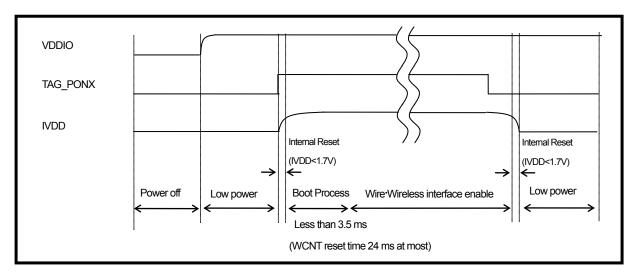
Figure 6-1 Timing of reset releasing and reset in TAG.
