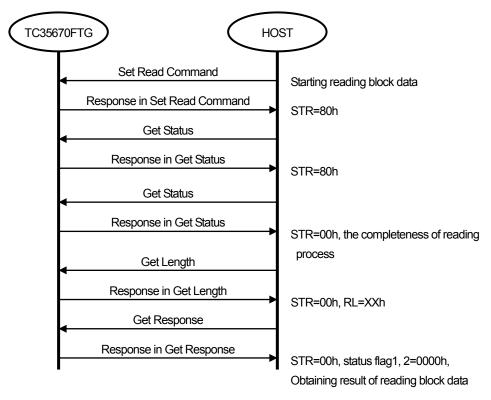
Figure 4-23 Operating sequence over the wired interface (Get Status/Get Length are used)
