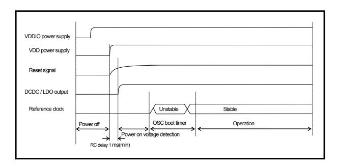
Figure 4-2 Power-on reset release sequence
