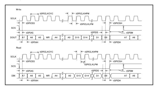
Figure 9-4 SPI Interface timing diagram
