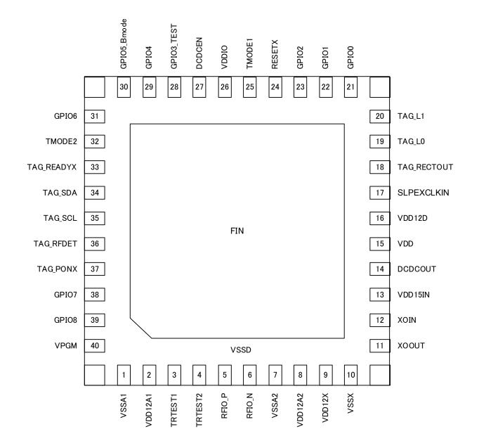
Figure 2-1 Pin Assignment (Top View)
