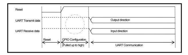
Figure 4-4 UART function assignment
