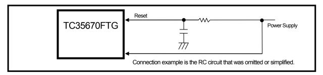
Figure 4-1 Reset signal connection example
