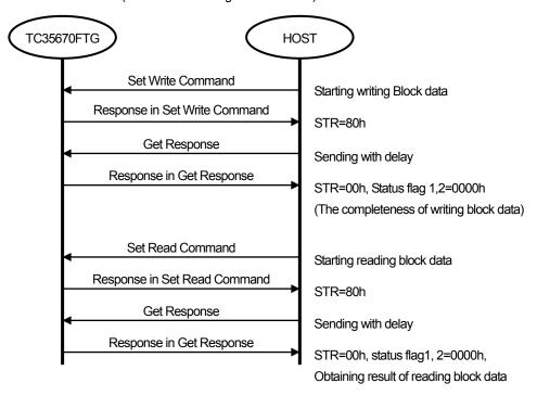
Figure 4-22 Operating sequence over the wired interface(Get Status/Get Length are not used)
