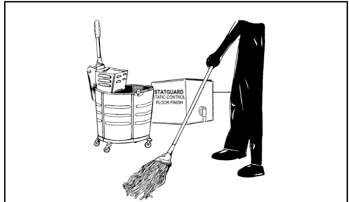
Figure 7. Applying floor finish
