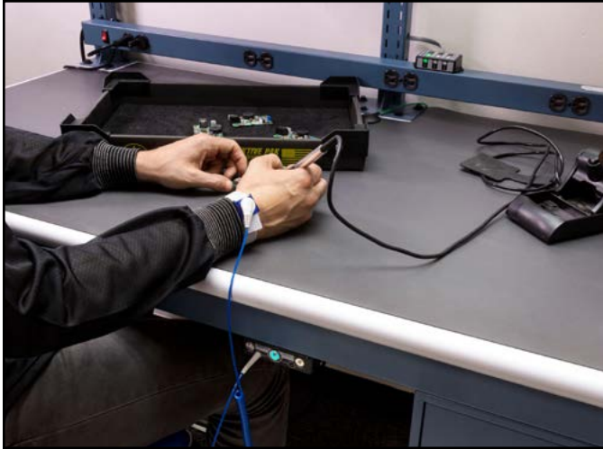
Figure 9. Using the Dual Operator Continuous Monitor at a one-person workstation
