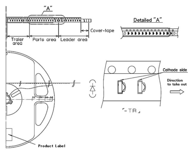
Note "-TR" means cathode side of LEDs should be placed on the sprocket-hole side.
