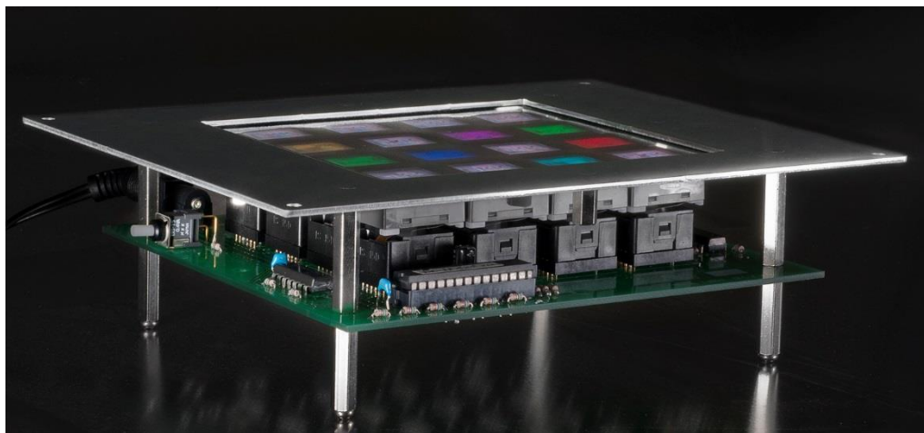
Photo of Overlay with switches and bezel
