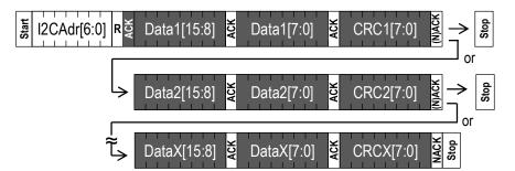
Dark areas with white text indicate that the sensor controls the SDA (Data) line.
