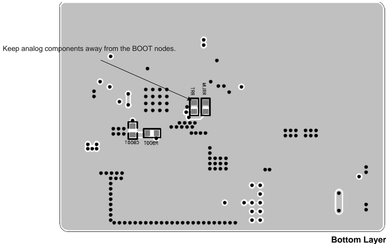
Figure 31. Layout Guide (Bottom Layer)
