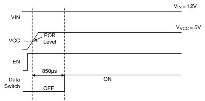
Figure 6. Data Switch On Sequence
