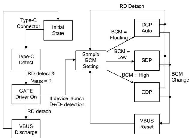
Figure 26. Detection Flow
