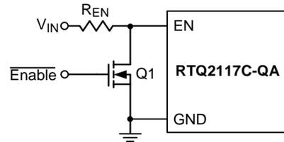
Figure 22. Logic Control for the EN Pin
