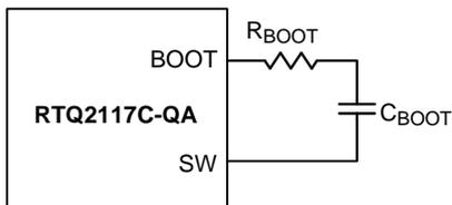
Figure 19. External Bootstrap Resistor at the BOOT Pin
