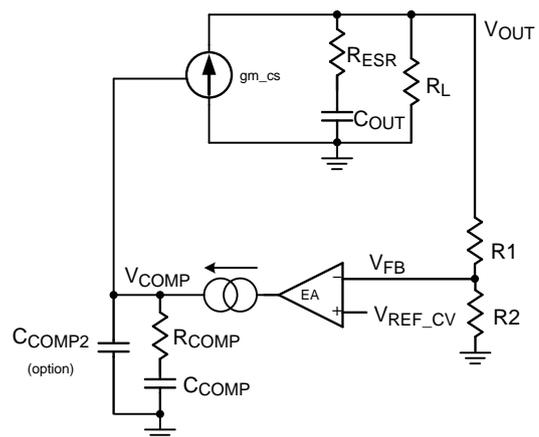
Figure 16. Simplified Equivalent Circuit of Buck with PCMC
