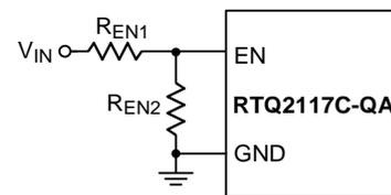
Figure 23. Resistive Divider for Under-Voltage Lockout Threshold Setting
