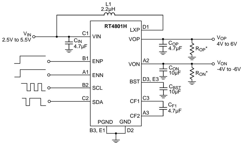
\* : R<sub>OP</sub> And R<sub>ON</sub> should be paralleled with V<sub>OP</sub> and V<sub>ON</sub> if output continuous discharge is required when channel is powered off.
