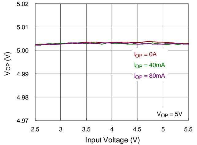
V<sub>ON</sub> vs. Input Voltage
