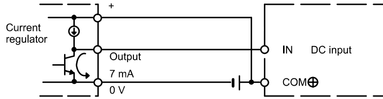
NPN open-collector output
