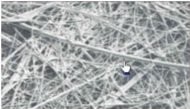
Photomicrograph of the fiber weave of a SCS filter (500x)
